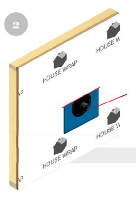
Slide the Quickflash® panel up underneath the WRB and over the penetration pressing down firmly to ensure a flush seal.
