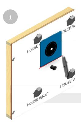
Using the Quickflash® panel as a guide, mark the length of the panel plus 1/4" on each side 2" above penetration onto the WRB and using a utility knife, cut a slit along the mark.
