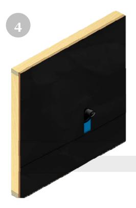
Install the weather resistant barrier carefully cutting an opening around the protruding pipe, over the top of Quickflash® panel using shingle style method extending to the bottom of flashing panel or further down.
