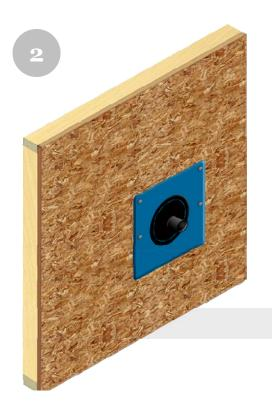
Using non-corrosive fasteners, secure the Quickflash® panel to the structure from the midpoint of the panel to the top.
