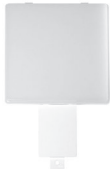
(1) 10 Watt Dimmable LED chip panel/3000 Kelvin Warm White/90CRI/700 lumens/70 LPW/ ENERGY STAR 2.0 certified/50,000 hours rated average life /<1W LED night light.
