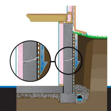
DELTA®-MS bridges cracks.... Water stays outside.
